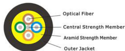
Distribution tactical fiber optic cable
