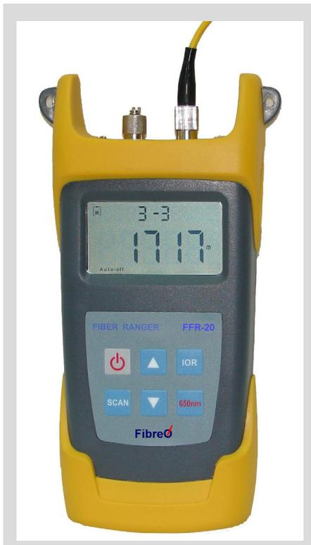
FibreOptica's Fiber Ranger uses the same work principal as OTDR. Therefore, the Fiber Ranger can also be treated as simplified, non-curve displayed OTDR. FFR-20 series are designed for the identification of fiber break point and fault locations. It can quickly detect and identify fiber break and impairment in fiber installation and display the results - up to 8 points.
