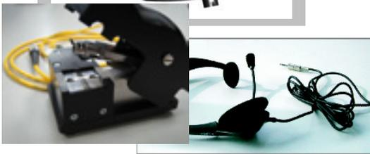
FTS-20 is a multifunctional fiber talk set consolidating with full-duplex talk set, stable laser sources, a tone generator and a detector. Its built-in steady laser sources can be used as regular ones to meet needs. It provides high-quality voice communication over a single fiber; it also supports three-way communication.
