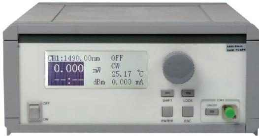
The JWD-1100 series high stable light source are microprocessor controlled laser diode sources which can support the variety of emitters such as: DFB, FP, PUMP, SLED and etc. It is specially used in passive components testing, power meter calibration and general laboratory uses.
